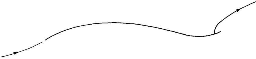
FIGURE 2. Kutta condition satisfied at the leading edge but not the trailing edge.
